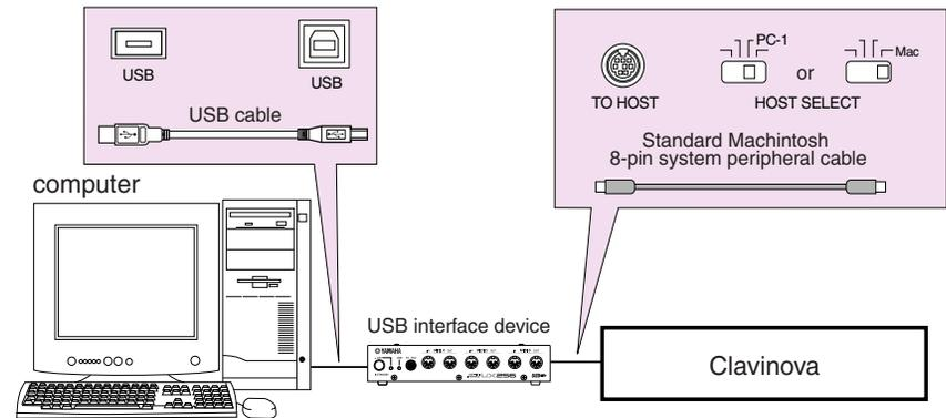
Using a MIDI cable to connect a USB interface device and the Clavinova:
