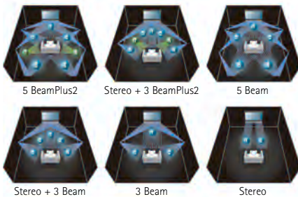
YSP-5100 includes 40 beam drivers, two woofers, two tweeters and a digital amplifiers
