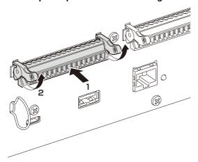
2. To disconnect Euroblock connectors, lower the left and right locks and pull out the connector.
