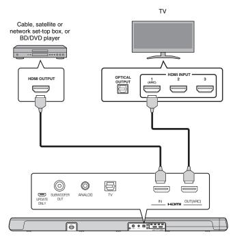
When a TV that supports Audio Return Channel (ARC) will be connected, the sound bar can only play audio from the TV when it is connected as shown above.
