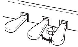
Rotate the adjuster until it comes in firm contact with the floor surface.
