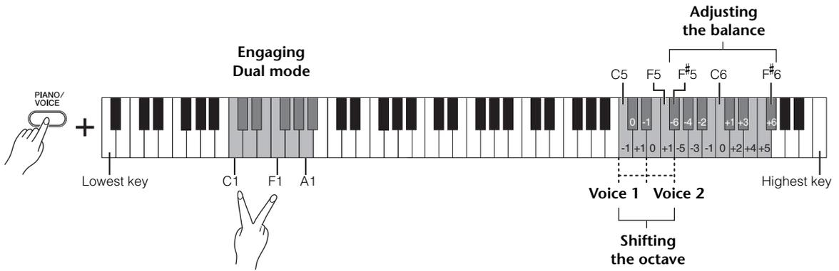
The Voice assigned to the lower key will be designated as Voice 1, and the Voice assigned to the higher key will be designated as Voice 2. You cannot assign the same Voice to both Voice 1 and Voice 2 simultaneously in Dual mode.
