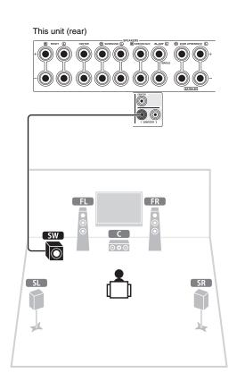
Use an audio pin cable to connect the subwoofer ( SW ).
