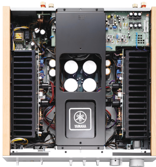
Completely symmetrical left-right construction.
