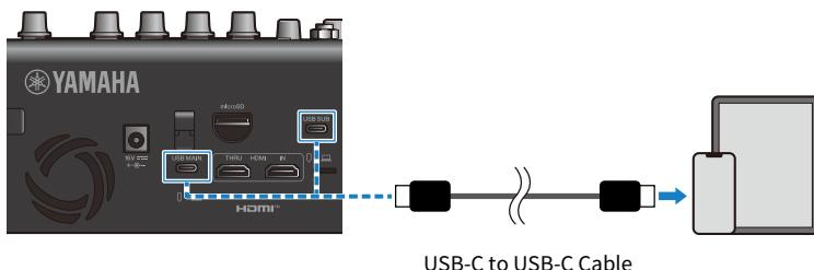
This product is automatically recognized by the iPad, iPhone or Android device once connected.
