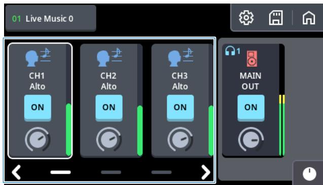
Touch the buttons aside from the ON button or the level knobs to select them. Touching a selected channel again shows the “Channel view screen” (p.125).
