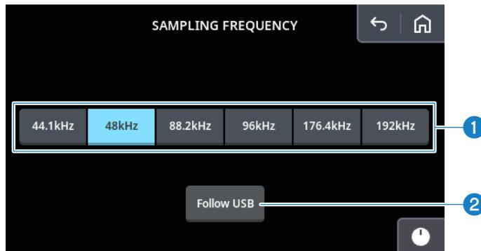
① **[44.1kHz, 48kHz, 88.2kHz, 96kHz, 176.4kHz, 192kHz] buttons**
