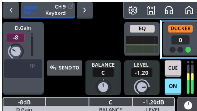
Touch the DUCKER button to switch it on/off. Use the [TOUCH AND TURN] knob to set the threshold.
