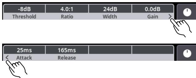
When USER DEFINED KNOBS mode is on, you can control the value of the parameter you set. Touch [<<] or [<>] to switch between the four banks (1–4) of the USER DEFINED KNOBS. The selected bank number is outlined in the illustration below.
