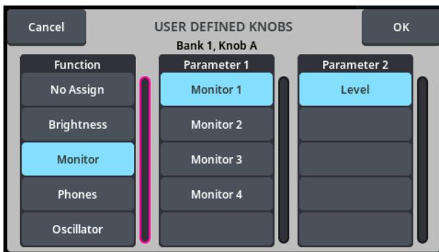
Abbreviations of the selected Function names and Parameter names are shown at the bottom of the screen when the USER DEFINED KNOBS mode is turned on.
