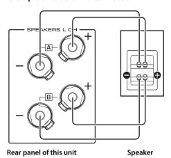
3 Set the SPEAKERS selector on the front panel to A+B BI-WIRING.
