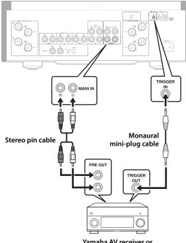
Yamaha AV receiver or other component that features TRIGGER OUT jacks and PRE OUT jacks
