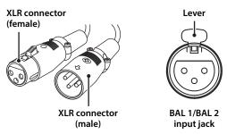
For a balanced connection, select BAL 1 or BAL 2 as the input source.
