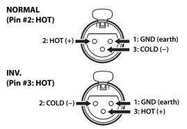
Refer to the instruction manual for the connected component to find out the position of the HOT pin at the balanced output jacks on the component.
