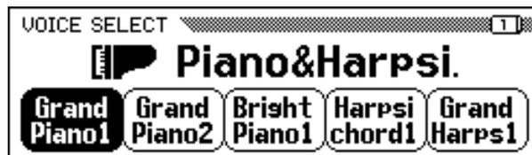
When you press one of the VOICE buttons, the LCD displays a new set of functions listing the voices of that type. You should now be looking at a menu of piano voices.
