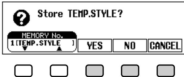
Select a memory number and press **YES** to store the style and exit, press **NO** to exit without storing the style, or press **CANCEL** to return to the Custom Style mode.
