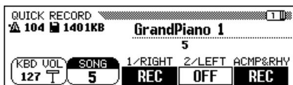
When a part is set to **REC** (recording enabled), the Synchronized Start function is set to stand-by, and recording automatically starts when you play the keyboard.
