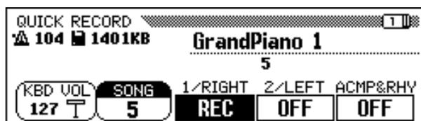
Call up page 1 by using the PAGE [◀] and [▶] buttons if the lamp is lit but the QUICK RECORD display is not shown.
