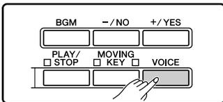
While holding down the [VOICE] button, press the highlighted keys shown below to change the settings of the Reverb effect and other keyboard functions such as Octave Shift and Dual balance.
