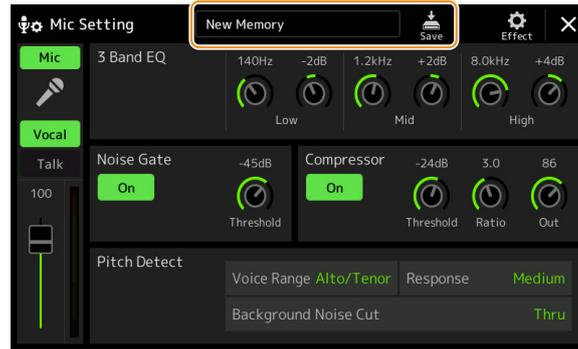
All the microphone settings can be saved as a single file by touching
