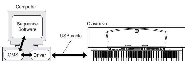
First install OMS before you install the USB-MIDI driver. Also, after installing the driver, you will need to set up OMS (above).
