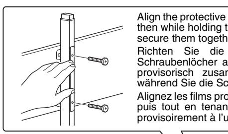
Align the protective sheets ⑤ with the screw holes, then while holding the sheets in place, temporarily secure them together with the pedal unit.
