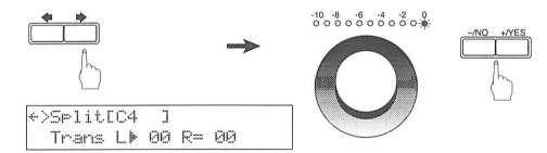
The MIDI output can be transposed from -60 to +60 in one semitone steps. Seperate transposition values can be set for the left- and right-hand parts.
