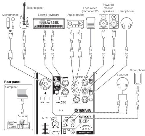
**NOTE** If you are using condenser microphones, turn on (\_\_) the [+48V] phantom power switch.
