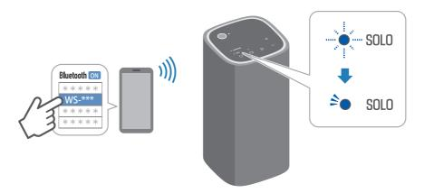
When the connection is established, the SOLO lamp glows blue.
