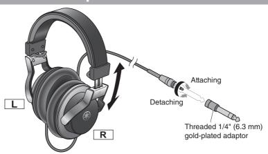
Wear the headphones with the L mark in your left ear, and the one with the R mark in your right ear. Depending on the device to be connected, use the supplied threaded 1/4" (6.3 mm) gold-plated adaptor as necessary.
