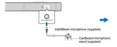
(PREPARATION & CHECK) ease connect the MIC. Please place the MIC at leas 8m/6ft away from Sound Proector. The MIC should be se ear level when seated. asurement takes about 3mii After [FNTFR] is pressed. please leave the room. [ENTER]: Start [RETURN]: Cancel
