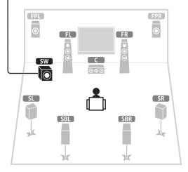
Use an audio pin cable to connect the subwoofer (SW).
