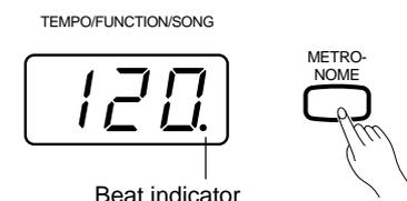
The metronome sound is alternately turned on and off by pressing the [METRONOME] button. When on, the beat indicator flashes at the current tempo.
