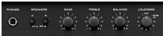
Flip-Down Hidden Control Panel offers headphone jack, speaker A, B or A+B selector, bass/treble/balance controls with center clicks and loudness control.
