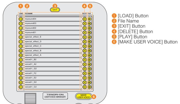
A graphic representation of the TENORI-ON and LED button arrangement in the Score Mode will appear on the display. [LOAD] buttons 1 through 16 on the display correspond to the equivalent TENORI-ON LED button positions.
