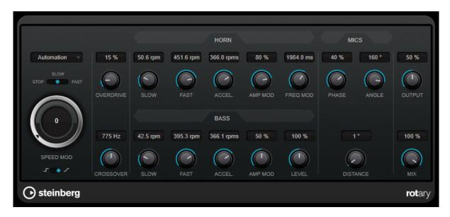
A rotary speaker cabinet features speakers rotating at variable speeds to produce a swirling chorus effect, commonly used with organs.
