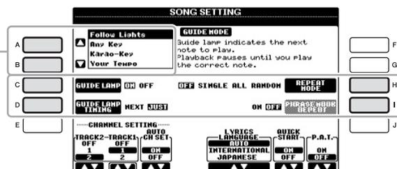
The [C], [D], [H] and [I] buttons are used to select the corresponding parameter.
