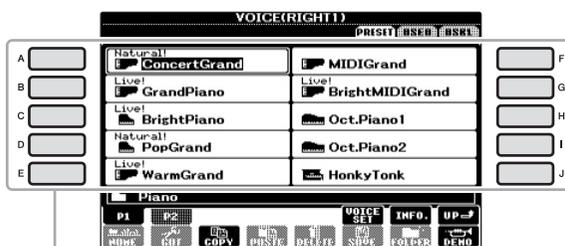
In the File Selection display (page 27), the [A] – [J] buttons can be used to select the corresponding respective files.
