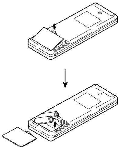
A diagram inside the battery compartment shows which way the batteries should be installed. Make sure you insert them correctly.
