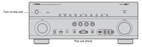
Before connecting the power cable (General model only) Make sure you set the switch position of VOLTAGE SELECTOR according to your local voltage. Voltages are AC 110-120/220-240 V. 50/60 Hz.
