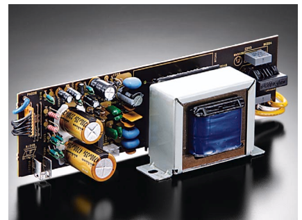
CD-1330 (MCS-1330 CD player) independent-structure power unit (top) and CD trans board (bottom).
