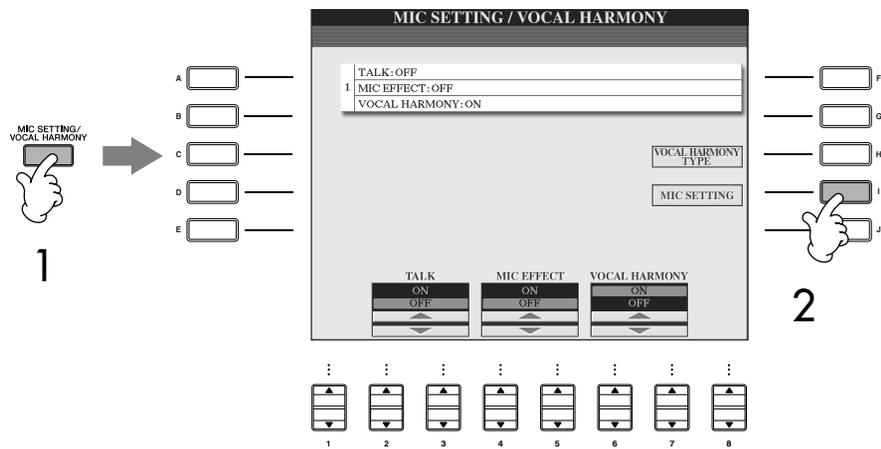
2 Press the [I] (MIC SETTING) button to call up the MICROPHONE SETTING display.
