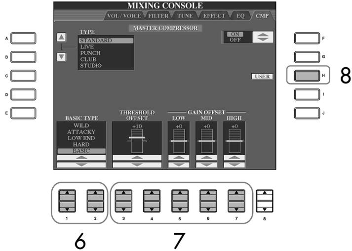
7 Use the [3 ▲ ▼]–[7 ▲ ▼] buttons to determine the Threshold (minimum level at which compression starts) and Gain (level of compressed signal at three separate frequency bands). These values offset those of the frequency curve settings in step 6.
