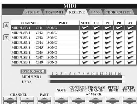
The explanations here apply to the RECEIVE display to be called up in step 4 of the “Basic Operation” on page 196. This determines which parts will receive MIDI data and over which MIDI channels the data will be received.
