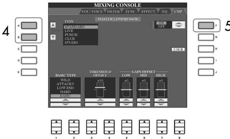
**5** Press the [F] button to set the Master Compressor to ON.
