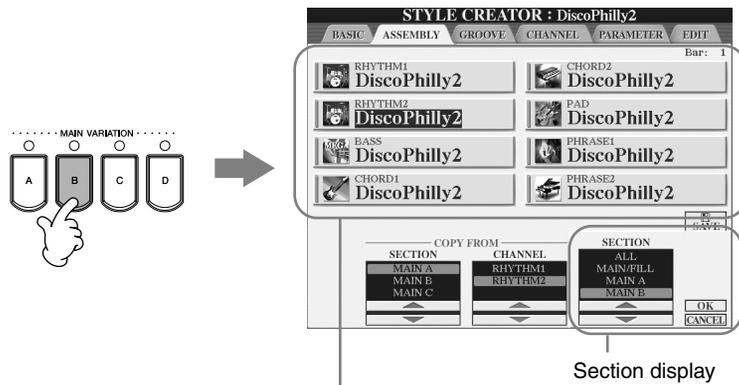
Indicates the channels that make up the section.
