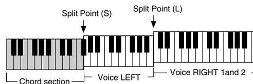
Press the [H] (S) button or the [G] (L) button and rotate the [DATA ENTRY] dial.
