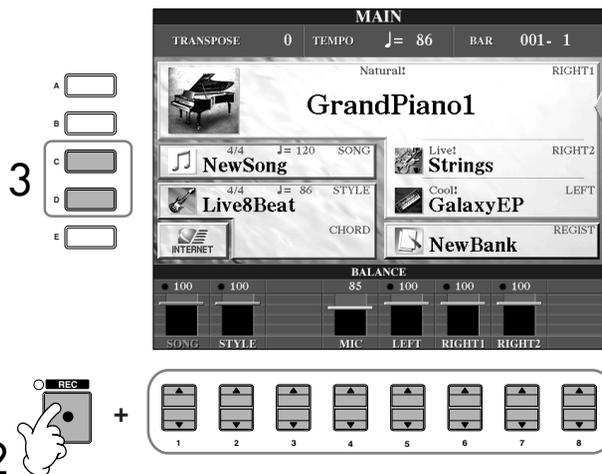
**3 Use the [C]/[D] buttons to select the desired part for the channel to be recorded.**
