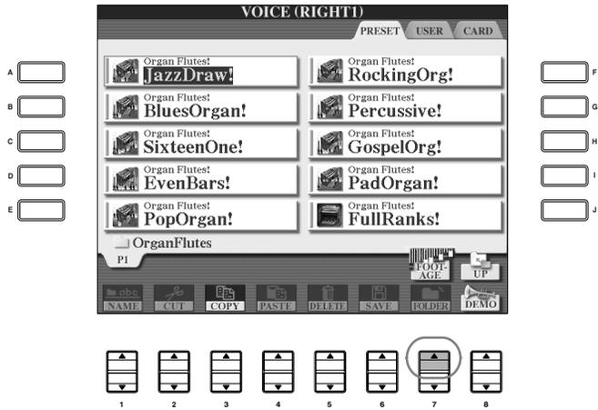
3 Use the TAB [◀]/[▶] buttons to call up the relevant setting display. For information on the available parameters, see the “Editable Parameters in the SOUND CREATOR [ORGAN FLUTES] displays” on page 99.
