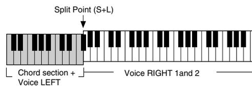
Press the [F] (S+L) button and rotate the [DATA ENTRY] dial.
