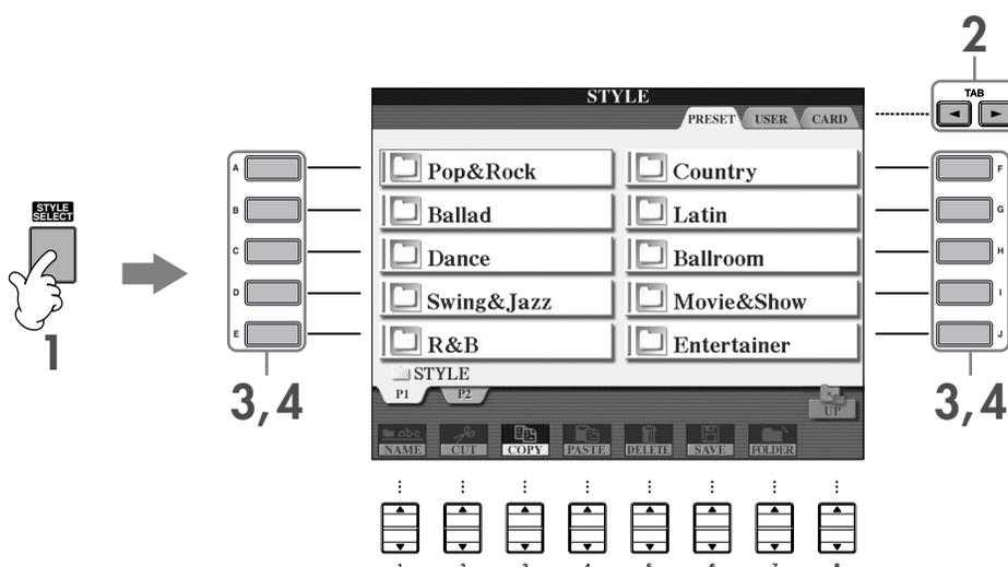
**2 Press the TAB [◀] button to select the PRESET tab.**
