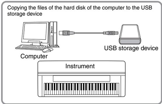
↓ Disconnect the USB storage device from the computer and connect it to the instrument
