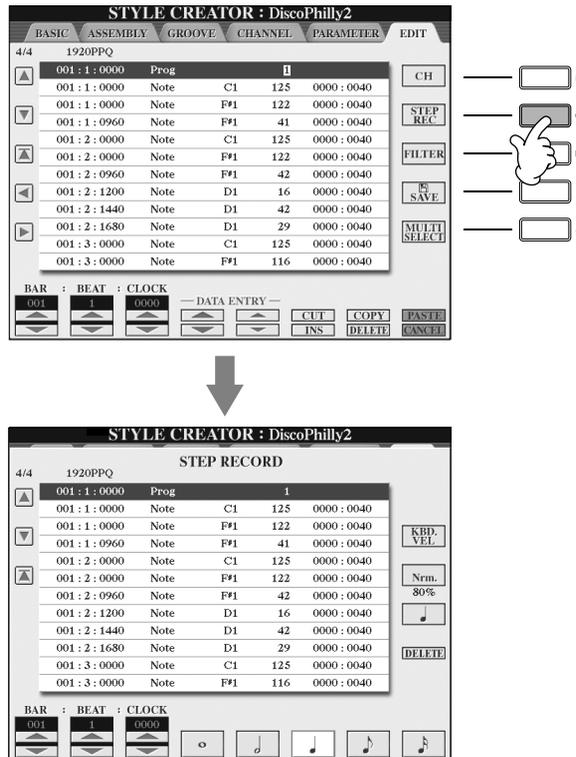
In the EDIT display, you can record notes with absolutely precise timing. This Step Recording procedure is essentially the same as that for Song Recording (page 115), with the exception of the points listed below:
