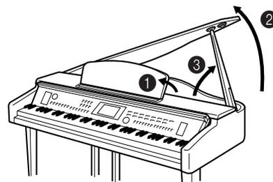
For the longer stay, use the inner recess, and for the shorter stay, use the outer recess to support the lid.
