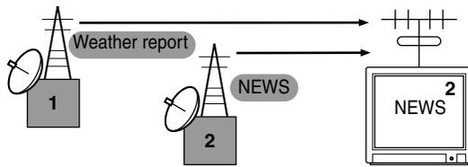
MIDI operates on the same basic principle. The transmitting instrument sends MIDI data on a specific MIDI channel (MIDI Transmit Channel) via a single MIDI cable to the receiving instrument. If the receiving instrument's MIDI channel (MIDI Receive Channel) matches the Transmit Channel, the receiving instrument will sound according to the data sent by the transmitting instrument.
