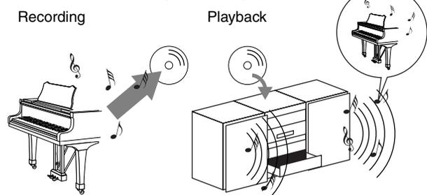
In the above example, the actual acoustic sounds of the pianist's performance are captured in the recording as audio data, and this is recorded to CD. When you play back that CD on your audio system, you can hear the actual piano performance. The piano itself is not necessary, since the recording contains the actual sounds of the piano, and your speakers reproduce them.
