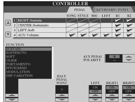
In addition to the footswitch or foot controller, the three piano pedals installed to the instrument (Right, Center and Left pedals) can also be assigned to various functions here. The following explanations cover the related operations and assignable functions (parameters).
