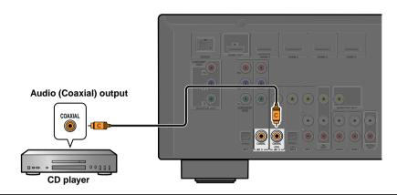
We recommend connecting audio devices with an coaxial digital output to the AV3 coaxial digital jack on this unit. This connection allows you to switch to the AV input 3 just by pressing the "CD" SCENE key (FSP. 26).
