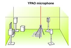
When positioning the microphone, we recommend that you use equipment that allows you to adjust the height (such as a tripod) as a microphone stand. When using a tripod, use the tripod screws to fix the microphone in place.
