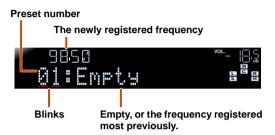
Press  $\boxed{5}$  PRESET  $\nearrow$  /  $\checkmark$  to select the preset to register the station to, and then press  $\boxed{5}$  MEMORY to register.
