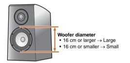
When speaker size is set to "Small," low-frequency components of the speakers that you configured are produced from the subwoofer (or from the front speakers if there is no subwoofer).
