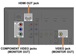
Video signals input from a particular type of jack(s) are output from the same type of jack(s). For example, these three output devices must be connected to the monitor by matching input/output jacks and cables, and then you must change the TV's input mode to the proper setting.
