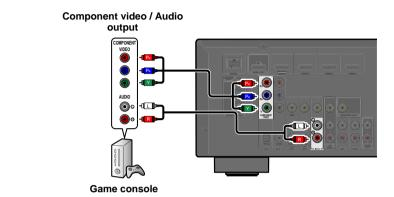
You can use the video input from the AV1-2 jacks in combination with the audio input from other AV inputs or AUDIO1-2.
