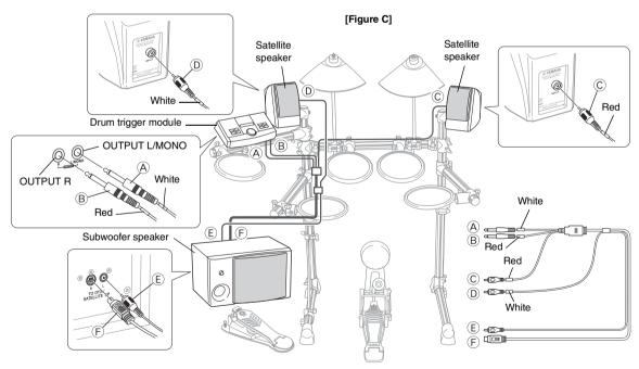
\* For the stereo audio cables, red indicates the right channel, and white indicates the left.
