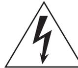
The lightning flash with arrowhead symbol within an equilateral triangle is intended to alert the user to the presence of uninsulated “dangerous voltage” within the product’s enclosure that may be of sufficient magnitude to constitute a risk of electric shock to persons.
