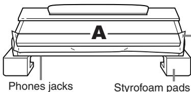
To prevent the key cover from accidentally opening during assembly, press down on the key cover, making sure that the sheet (shown) remain in place.
