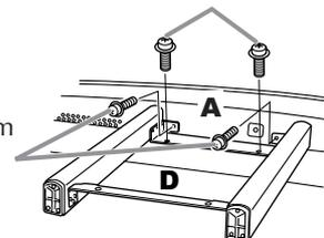
If the screw holes do not align, loosen the other screws and adjust the position of D.
