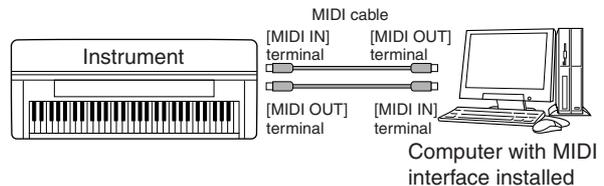
The second connection possibility involves a separate, external MIDI interface connected to the computer via a USB port or a serial port (modem or printer terminal). Using standard MIDI cables, connect the MIDI OUT terminal of the external interface to the [MIDI IN] terminal of the instrument, and connect the [MIDI OUT] terminal of the instrument to the MIDI IN terminal of the interface.
