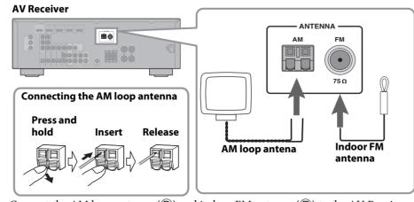
Connect the AM loop antenna (①) and indoor FM antenna (②) to the AV Receiver, as shown. See the owner's manuals for more information about connecting antennas.
