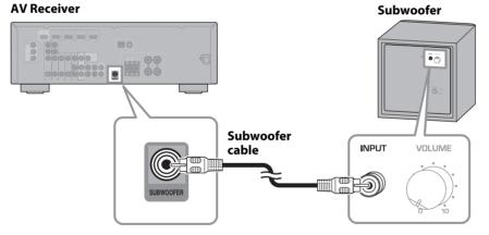
Use the included subwoofer cable (①) to connect the Subwoofer's INPUT jack to the AV Receiver's SUBWOOFER jack.
