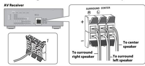
Connect the center speaker (H) and surround speaker (G) cables to the AV Receiver. Make sure you connect the speakers with the correct polarity—positive (+) terminals to positive (+) terminals, and negative (-) terminals to negative (-) terminals.
