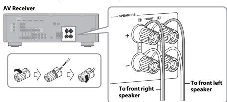
Connect the front speaker (⑤) cables to the AV Receiver. Make sure you connect the speakers with the correct polarity—positive (+) terminals to positive (+) terminals, and negative (-) terminals to negative (-) terminals.
