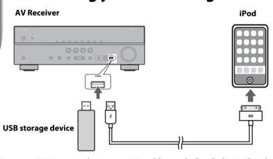
Connect a USB storage device or a USB cable supplied with the iPod to the AV Receiver's USB jack (on the front panel), as shown.
