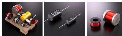
Woofer crossover network (left), Solen metalized polypropylene capacitors (centre) and large iron-core coil (right)
