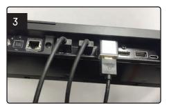
Connect HDMI cables to correct inputs/outputs on the Sound Bar.
