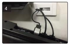
Use flexible, thin HDMI cables and/or 90-degree adaptors.
