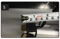
Depth of HDMI plug should not exceed 25 mm (refer picture).
