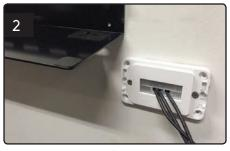
Run cables. In this example, cables are run through a wall plate.
